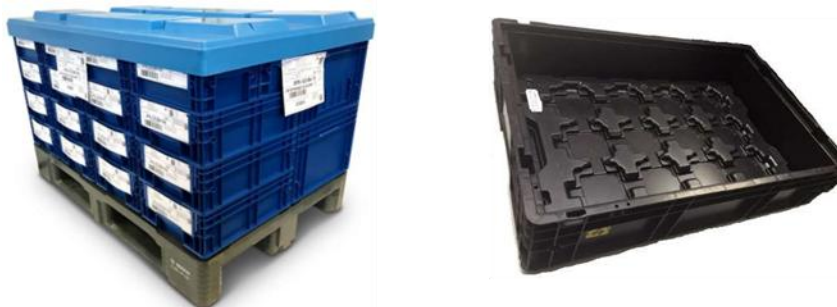
Figure 25: Pallet with crates (left) and crate with blister (right)
